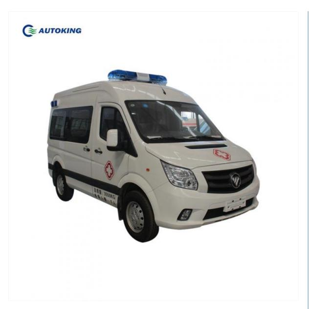
The exterior design of the Foton G7 ambulance features red or blue reflective strips. The driver's door, hood, and tailgate display reflective rescue logos for high visibility. The medical cabin includes glass windows with frosted glass paper covering 2/3 of their height, ensuring privacy while allowing natural light penetration.
